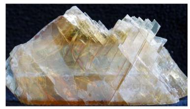
Sheetrock is made out of gypsum (calcium sulfate dihydrate) which is mined from the ground.
